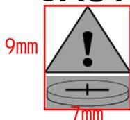
This symbol marked on the product indicates "Warning:contains coin battery". 2.5mm
